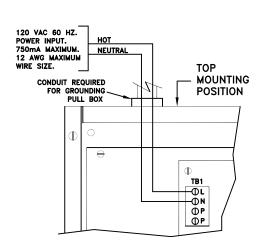
GENERAL WIRING DIAGRAM FOR 2901 ELECTRIC LATCH RETRACTION CONTROLLER
